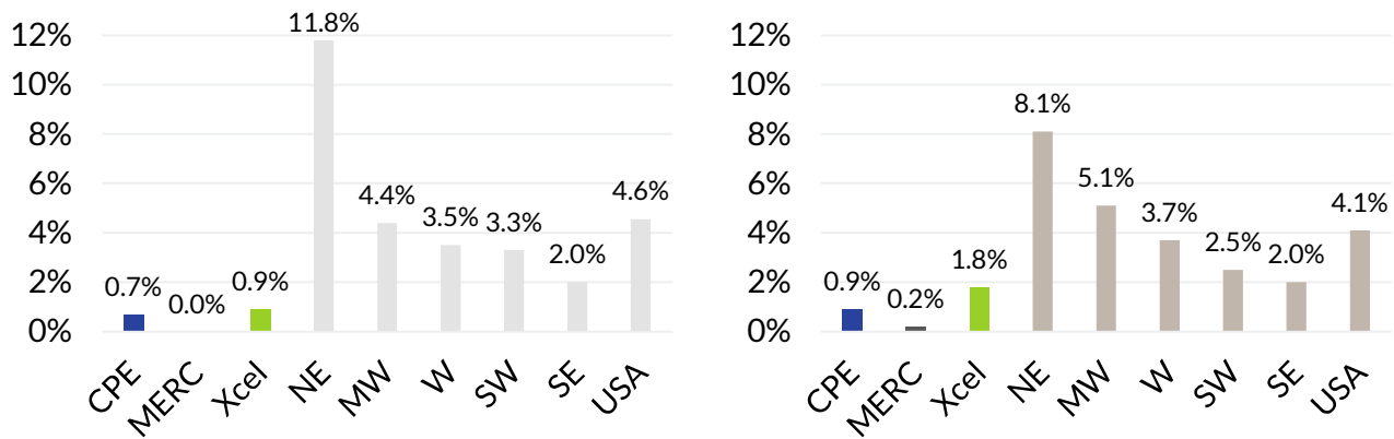
Figure 1.4: Composition of Leak-Prone* Mains (Left) and Services (Right) by Utility and Region, 2022
